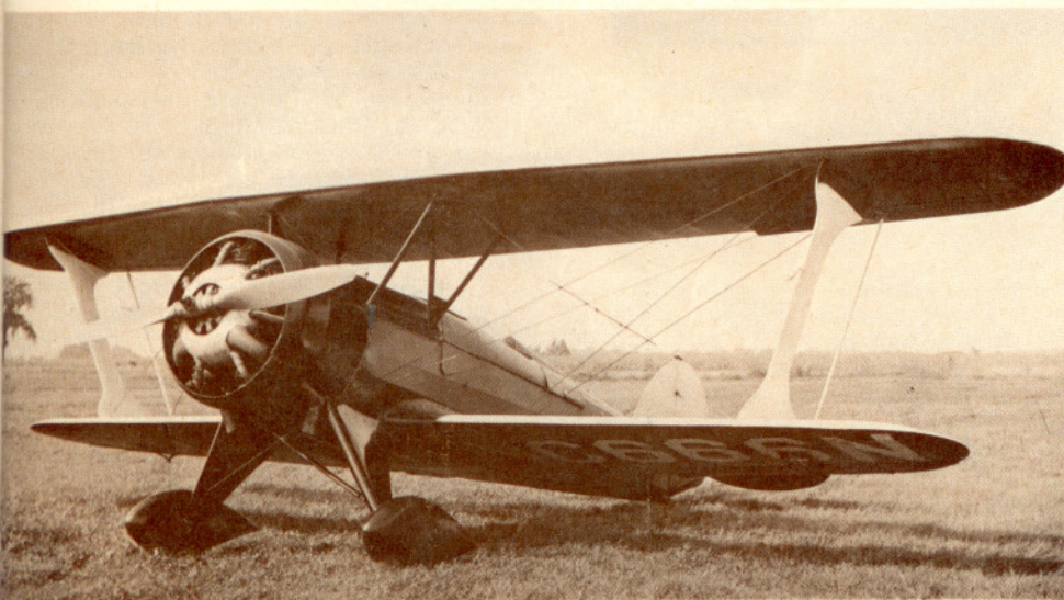
The 1929 CTO Taperwing used the 225 h.p. Wright J-6-7 engine. This one, owned by Art Davis, was modified for racing by the addition of a speed ring around the engine and the substitution of special low-drag struts and landing gear for the originals.
